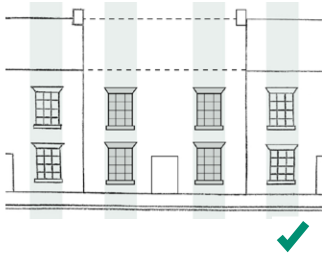
Figure 73: Good practice diagram: the window typology and fenestration pattern match the ones of neighbouring properties
