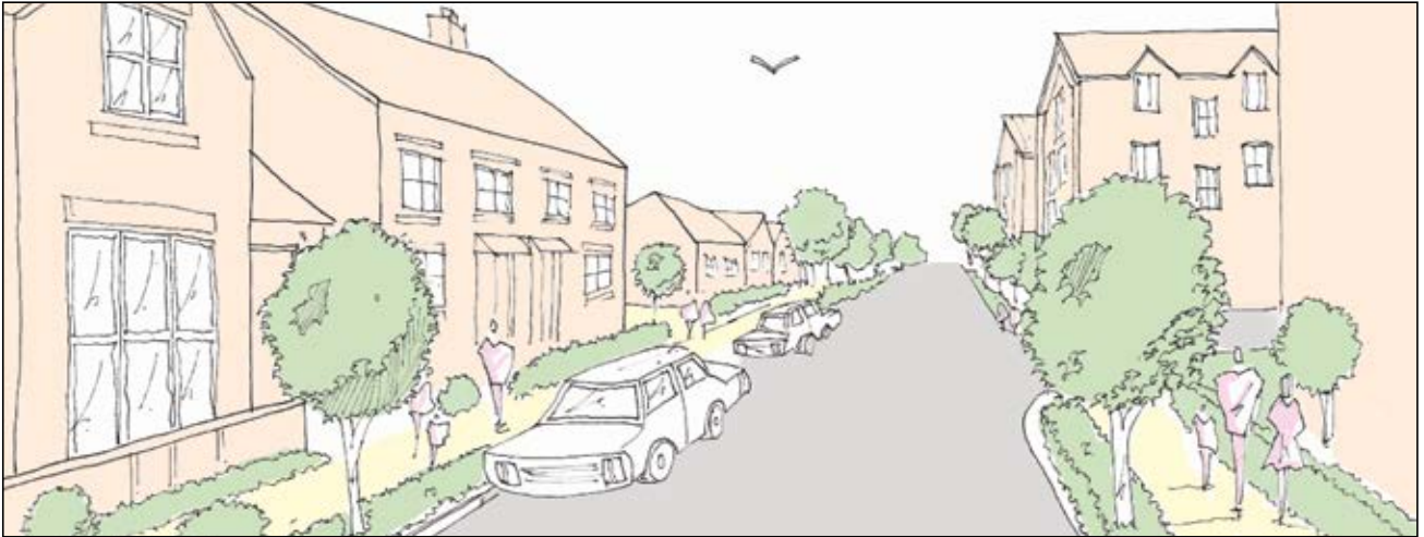
Figure 79: Improve on street parking by designing bays that are broken up by planting, rain gardens and streets trees.
